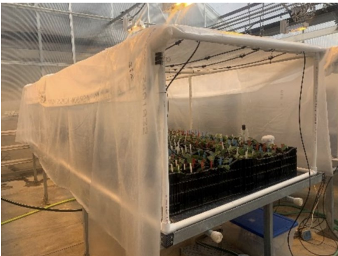
Figure 2. Sample misting chamber, 14' long x 5' wide x 3' tall. (Image from Shrestha and Miles 2023.)
